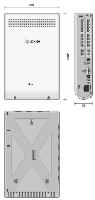
Figure 2.2.2 KSU exterior and dimension
